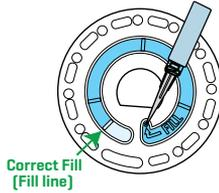
2. Do not overfill the disk. If the disk is overfilled, sample water will flow out of the overflow hole in the center of the disk. The disk is not leaking. Dry the disk and run the test.
