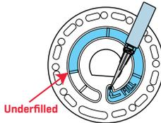
4. Do not introduce air bubbles into the disk. The reagent chambers will not fill entirely and results will be inaccurate. As soon as a bubble starts to form, pull back on the plunger to draw the bubble out of the disk. Begin the filling process again.
