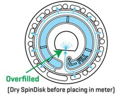
3. Do not under fill the disk. If the disk is under filled, the reagent chambers will not fill entirely and results will be inaccurate.
