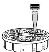
2. Do not overfill the disk. If the disk is overfilled, sample water will flow out of the vent hole in the center of the disk. If this happens sample water may flow into a reagent chamber prematurely and results will not be accurate. Begin a new test in the next chamber.
