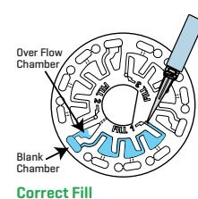
3. Do not under fill the disk. If the disk is under filled, the blank chamber will not be full. The reagent chambers will not fill entirely and results will be inaccurate.
