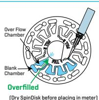
4. Do not introduce air bubbles into the disk. The reagent chambers will not fill entirely and results will be inaccurate. As soon as a bubble starts to form, pull back on the plunger to draw the bubble out of the disk. Begin the filling process again.
