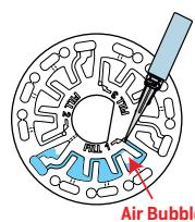
6. Disks should be filled and used within 10 minutes. They cannot be filled ahead of time.
